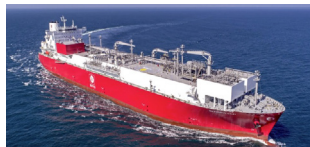
A 170,000 m 3 -class vessel delivered in 2020 and converted into an LNG-FSRU
